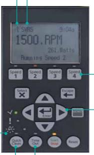
Function buttons to set speeds for separate operations—filtration cycles, spas, cleaners, water features and more
