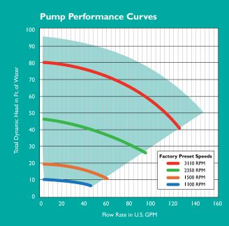
NOTE: The chart above demonstrates performance rates at factory preset speeds of 1100 RPM, 1500 RPM, 2350 RPM and 3110 RPM. However, flow rates can also be custom programmed between the ranges of 1100 RPM and 3450 RPM as indicated by the green tint.
